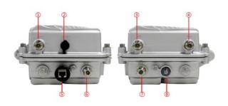
MESH Antenna Interface Power Input Port - DC 12V WIFI Antenna Interface MESH Antenna Interface LAN Interface - RJ45 Antenna Interface - Reserved Antenna Interface - Reserved Signal Indicator
