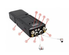
Main body power input port HDMI input (mini HDMI interface) WIFI antenna interface LAN input interface (9-pin LEMO connector), pin-1234 equals RJ45 pin-1236 (Tx+, Tx-, Rx+, Rx-), and Pin-5678 equals RJ45 pin-1236 (Tx+, Tx-, Rx+, Rx-). Mic input interface GPS/BD antenna interface MESH antenna interface-1 Power push button Signal Indicator SNR Link Quality Topology Color SNR ≥ 17 Excellent Deen Green
