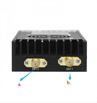
a. ANT2 Port - Auxiliary antenna, works as auxiliary receiving, NO transmitting. b. ANT1 Port - Main antenna, work mode is TDD transmitting/receiving.
